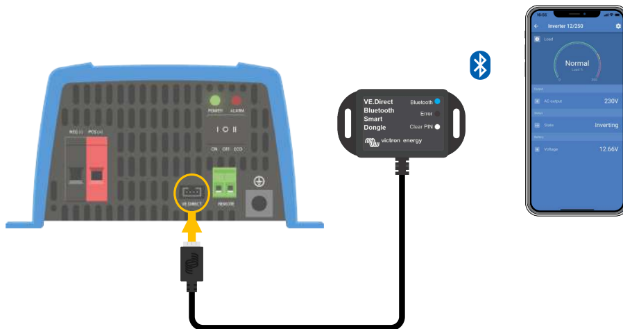
Connection drawing VE.Direct Bluetooth Smart Dongle
