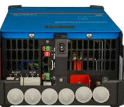
MultiPlus 2000 VA (bottom cover removed)
