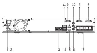
1 Power Switch Power Input Network Ports **USB Ports** AUDIO IN, RCA Connector HDMI Ports 6 RS-232 Port 8 Alarm In/Out 10 AUDIO OUT, RCA Connector 9 VGA Ports
